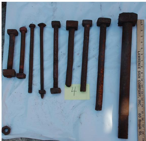
Some bolts were used to fit in a slot on a machine, or a sluice gate control, to lock it in place. Square headed bolts were the norm because they were easier to produce and work with. Today bolts of this nature are hexagon. When you turn a hexagon bolt with a hexagon wrench you turn it 60 degrees. When you turn a square bolt with a square wrench you had to turn it 90 degrees. This was a more difficult and less efficient process.
